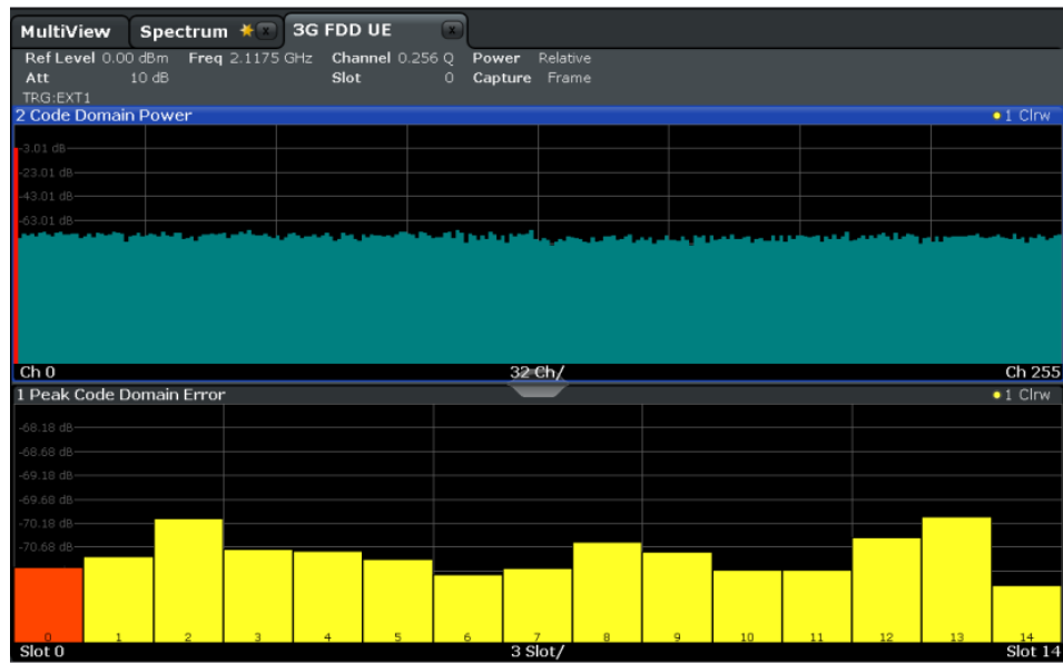
Fig. 10-8: Measurement Example 6: Determining the Peak Code Domain Error
