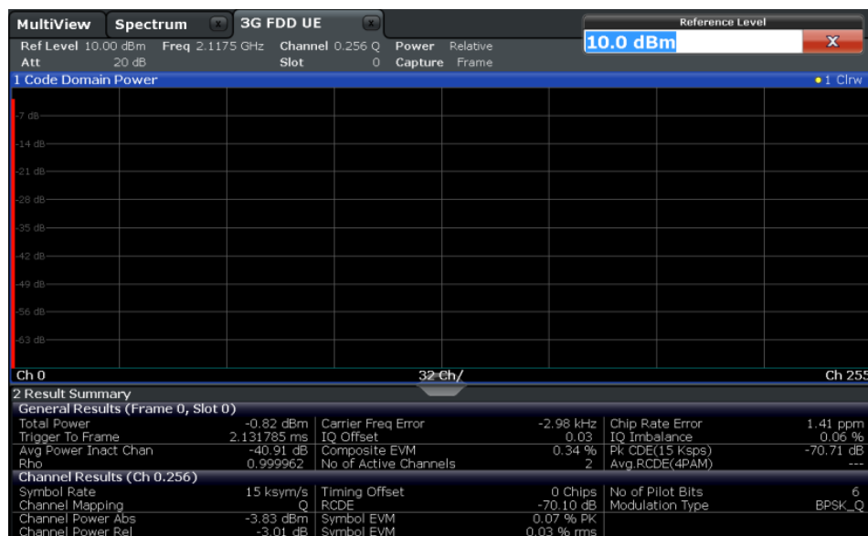
Fig. 10-3: Measurement Example 3: Measuring the Relative Code Domain Power
